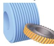
Bulk production of gears with a small to medium module is most productive with a continuous generating gear grinding process.
