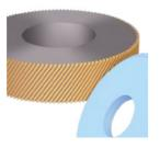
If you grind gears with large modules or in small quantities, profile grinding is the perfect solution.
